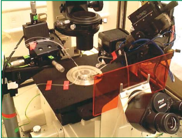
Apparatus used for monitoring the tiny electrical voltages that occur at synapses.
