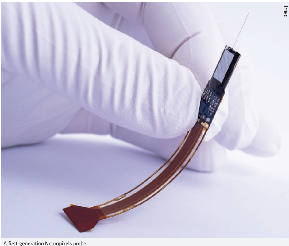
A first-generation Neuropixels probe.
